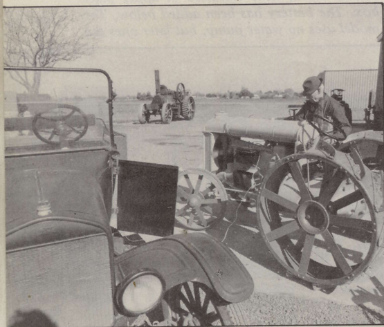
Above: Hotspot on intake manifold allowed Fordson to burn kerosene. It started on gasoline, then switched over after warming up. Below: Heidrich, of Woodland, Calif., owns a large collection of farm machinery plus several cars, including this T roadster pickup.
