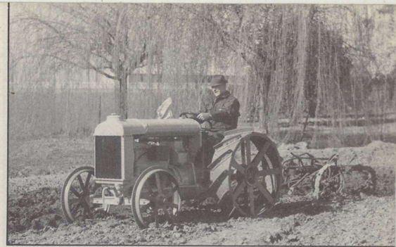
Above: Fred Heidrich demonstrates plow with his restored 1923 Fordson. If the plow hit a snag, it would tend to pull tractor over backwards. Later models had a gravity-weighted kill switch which helped prevent tipping. Below: A 1925 Fordson (foreground) shows off its fenders, also called "grouzers," which touched ground before tractor could rear over backwards. Bins in fenders provided storage for tools.
