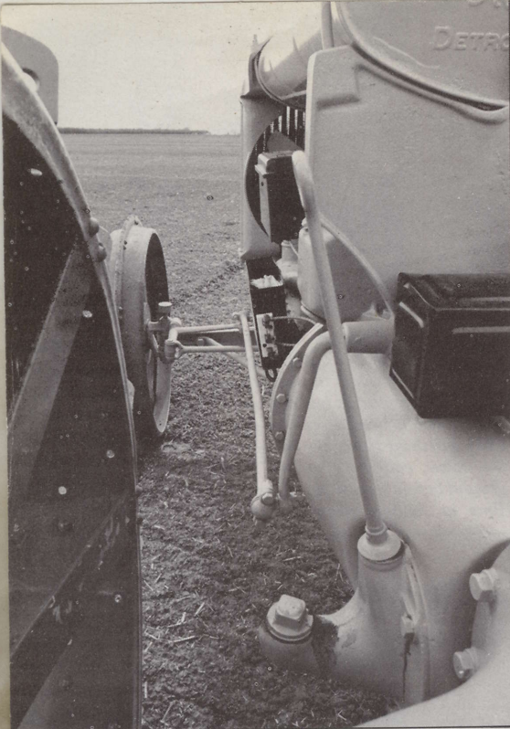
The Fordson shifts with left hand in an unconventional pattern. Unlike T, tractor used foot-pedal, multi-disc clutch and 3-speed transmission. Final drive was by worm gear.
